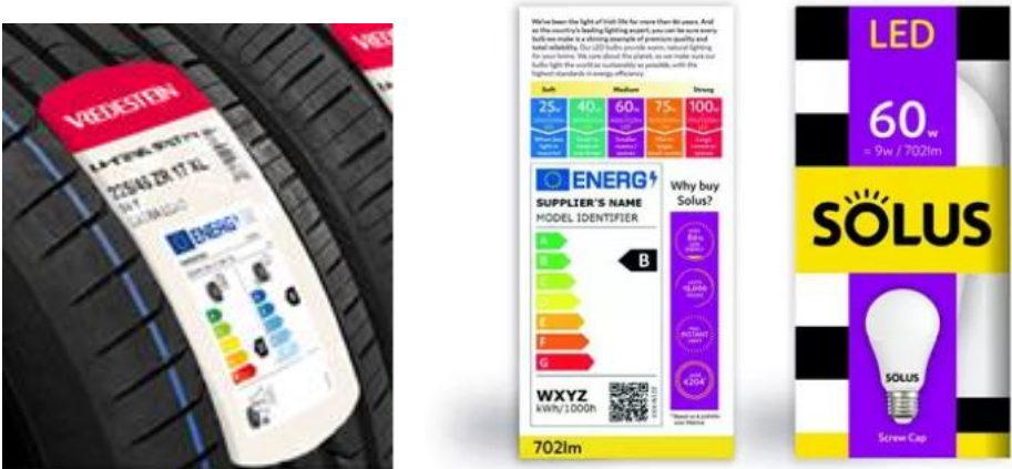
FIG. 2 EXAMPLES OF PRODUCT MODEL-LEVEL LABELS DEFINED BY THE ENERGY LABELLING REGULATION AND PLACED ON PRODUCT PACKAGE
